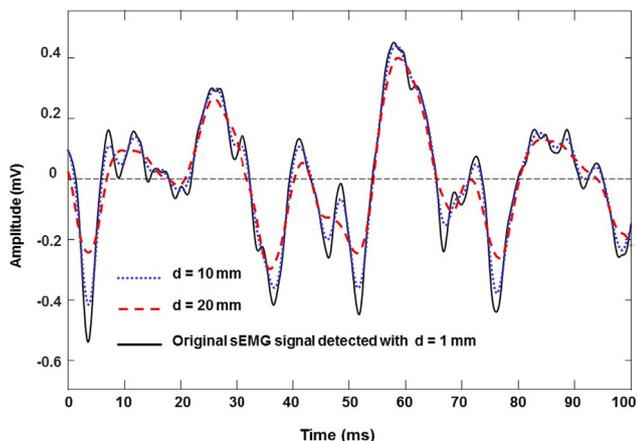
Fig. 12. Low-pass filtering effect for two different diameters of a circular electrode on a monopolar sEMG signal in time. The signal has been acquired with two pin electrodes having  $d = 1$  mm and has been filtered with the transfer functions depicted in Fig. 11. Observe the strong attenuation of the sharp peaks due to electrode size.
