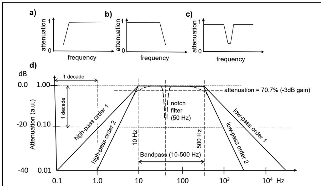
**Fig. 9.** Transfer function of analog or digital filters used for sEMG conditioning. a) high pass filter, b) low-pass filter, c) notch filter, d) combination of filters and concept of filter order. Note the logarithmic scales on both axes. A notch filter removes spectral lines of an undesired interference as well as spectral line of the sEMG signal that may be important See text for further explanation.
