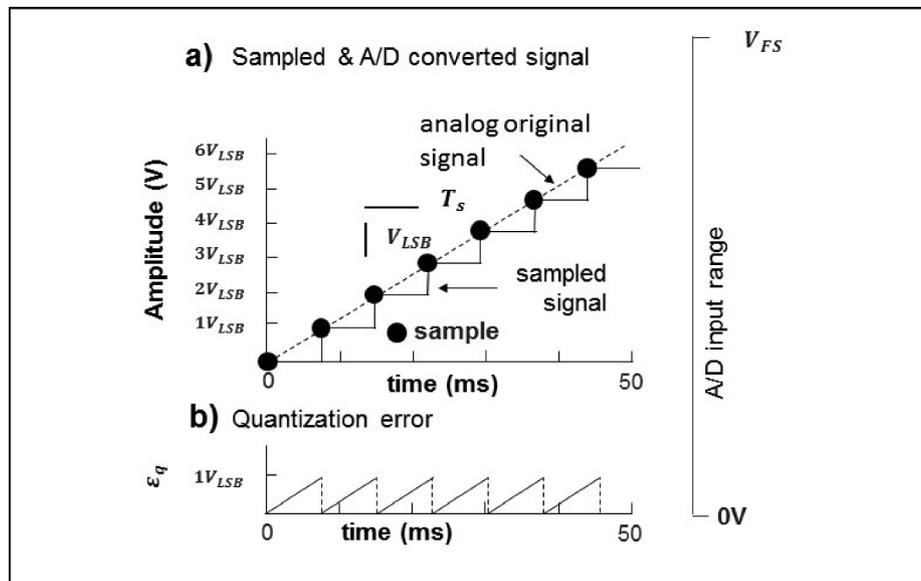
**Fig. 17.** a) Quantization error. A ramp signal is sampled (black dots) and converted (continuous black line) into a digital signal. b) The quantization error ( $\epsilon_q$ ), varies between 0 V (right after the conversion has occurred) and  $V_{LSB}$  (immediately before the new sample is acquired).
