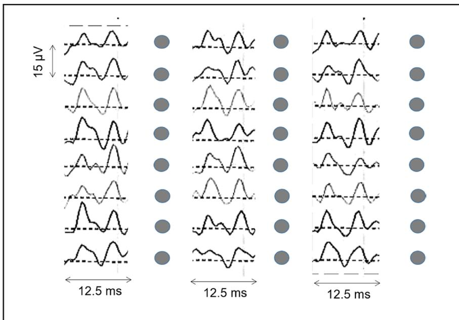
Fig. 4. Example of highly correlated noise across the monopolar channels of an 8x3 electrode grid applied on a piece of pig skin to avoid any sEMG contribution. This noise is reduced but not cancelled by the differential detection. Interelectrode distance = 10 mm in both directions, electrode diameter = 3 mm. Modified from (Russo and Merletti, 2017).
