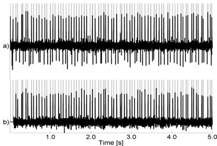
FIG. 3: IPT detected from synthetic surface EMG signals (10 active MUs, SNR = 10 dB) by a) BBS-based method (black), and b) IC-based method (black). Original IPT is depicted in grey.
