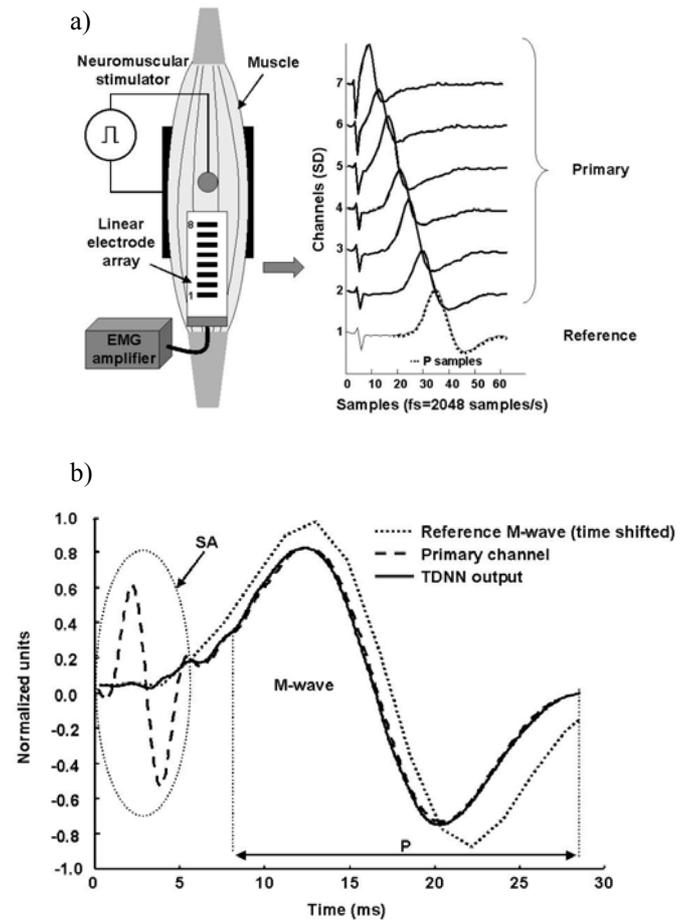
Fig. 1: Example of M-wave reconstruction using multichannel signal detection and processing. a) The compound action potential obtained from a channel (reference) of the array distant from the stimulation electrode was successfully used to estimate stimulus artifact (SA) and response and adaptively eliminate (using a Time Delay Neural Network) the first from the second even in channels (primary) closer to the stimulation electrode where overlapping between artifact and response is substantial.
