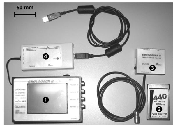
FIG. 2: The acquisition system, composed by: 1) the portable acquisition unit with graphical display interface and touchscreen; 2) a PCMCIA memory card; a 16-channel digital EMG probe; 4) an optional, optically isolated USB interface for online signal display on a PC.
