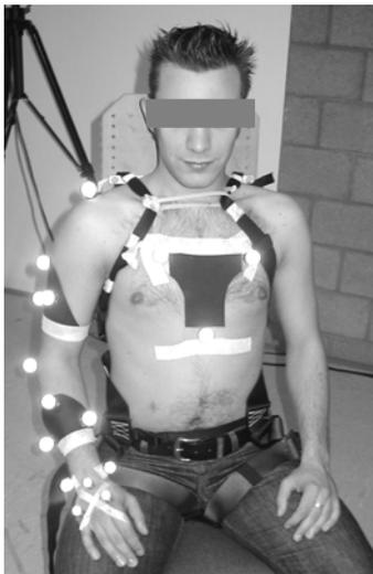
Fig 1: Marker triplets on body segments
