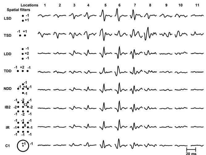
FIG. 3 : Single surface MU action potentials detected from the tibialis anterior muscle. The surface potentials were averaged using intramuscularly detected potentials as triggers. The results from 8 spatial filters are shown. The distance between each recording location is 5 mm, the inter-electrode distance of the point electrode spatial filters 5 mm and the radius of the ring system 5 mm. (From [12])
