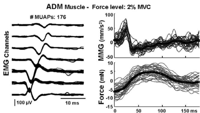
Fig. 2. Examples of single MU MMG and force signals for a representative contraction. The MMG and force response were obtained by averaging the signals following the occurrences of single MU action potentials used as triggers. All the detected occurrences in the 60 s long contractions were used for the averaging.
