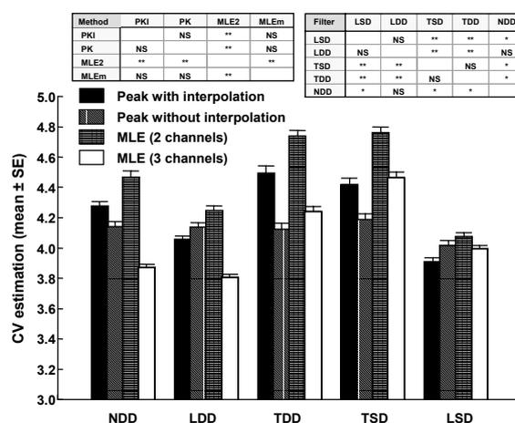
FIG. 2 : Influence of the choice of the spatial filter and estimation method on CV estimates. The methods compared were the estimation of CV from the peak delay with (PKI)
