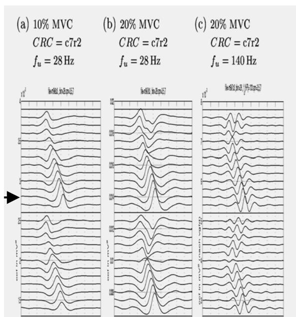
Figure 6: (a), (b) Cross covariance functions between bipolar SEMG channels which were measured at different load levels from the human biceps. The EMG channels were located in two columns parallel to the fibres. "→" is the covariance reference channel (CRC). (c) High pass filtered cross covariance functions.
