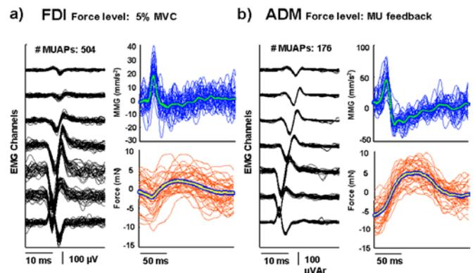
**Figure 1.** Single MU MMG and force signals. Spike triggered averaging on 60 s time window. Note the different MMG and force twitch response of the two muscles (redrawn from [4]).
