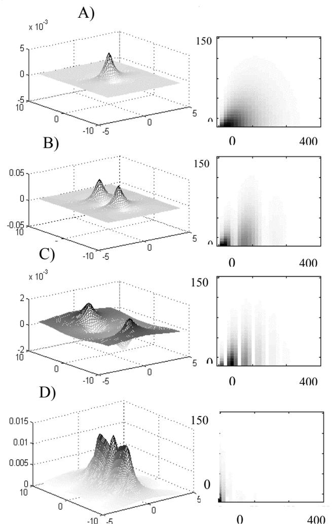
Figure 5: A) arising, B) travelling C) vanishing motor unit action potentials. and their spatial spectra. These spectra contain larger spatial frequencies than that of the RMS (D) of this action potential.
