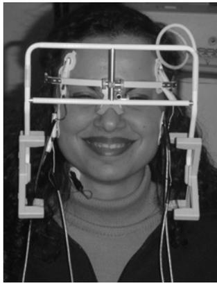
FIG. 1: Set-up of the Kinesiograph K6 and EM2 Myotronics in a young subject.
