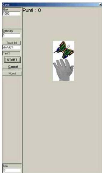
FIG. 2: Biofeedback set-up. The position of the hand image is a linear function of the level of myoelectric signal. Every time the subject succeeds in catching the butterfly it changes position alternating between zero and a randomly chosen position.
