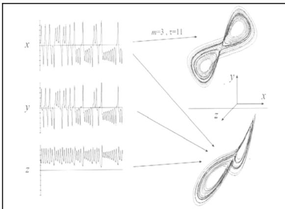
Fig. 6 : Reconstruction of an attractor using the delay coordinates method [4].
