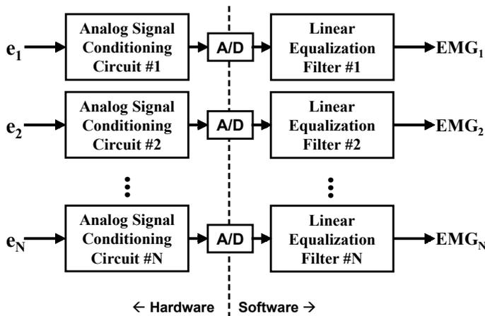
FIG. 1: Configuration of an EMG array system with channel equalization. Monopolar inputs  $e_i$  are conditioned by analog circuits [typically, a high-pass filter, selectable gain, electrical isolation and low-pass (anti-aliasing) filter]. The conditioned signals are analog-to-digital (A/D) converted. Each channel is then individually equalized via a software filter to form outputs  $EMG_i$ .
