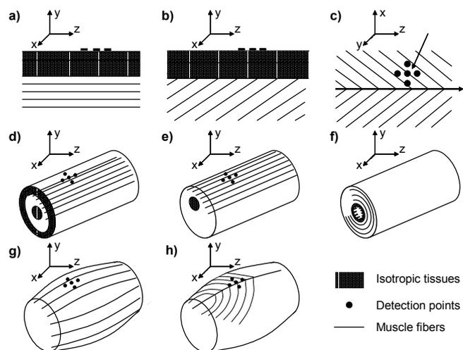
FIG. 1 : Examples of volume conductors. In some cases, both analytical and numerical solutions are available from the literature, while in others only numerical methods can be used. Analytical solutions exist for the cases reported in (a) [1], (b) [3], (c) [3], (d) [2], and (f) [2]. (From [4]).
