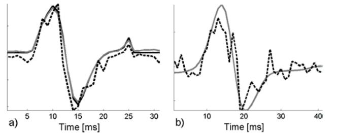
FIG. 2: The MUAPs identified by our BBS-based method (dashed) and the IC-based method (grey), from a) synthetic surface EMG signals (10 active MUs, SNR = 10 dB, original MAUP shape is depicted black-solid), and b) surface EMG recorded during an isometric 10 % MVC measurement of the right biceps brachii of healthy male subject (age 25 years, height 170 cm, weight 63 kg).
