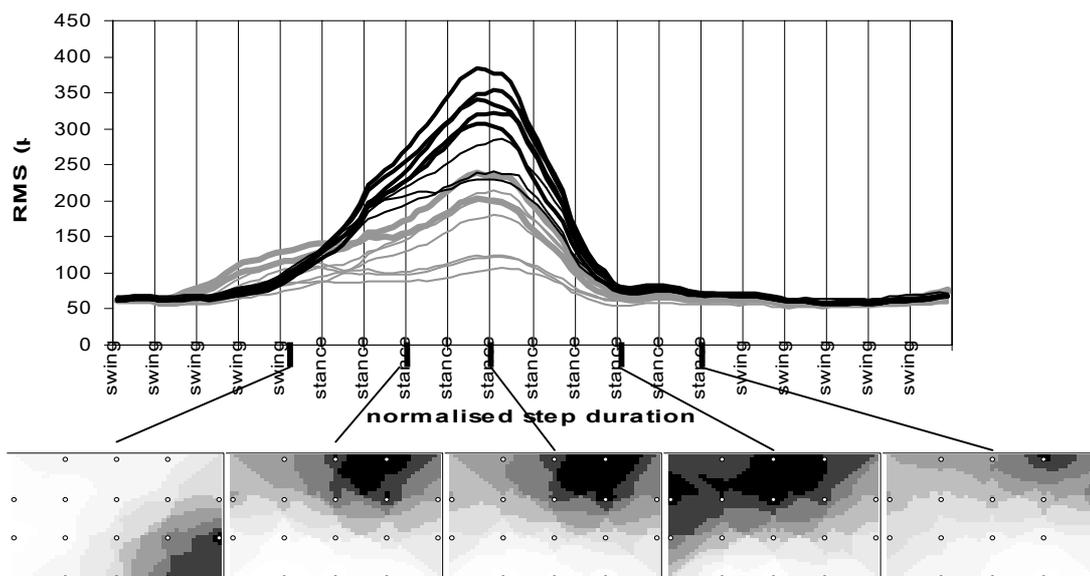
Figure 3: Time course of RMS from the triceps muscle of rats walking in a treadmill. The RMS map sequence clearly shows an inhomogenous activity distribution which depends on the phase of the movement. (These RMS values were calculated with a very short time window: 21ms., see [2])
