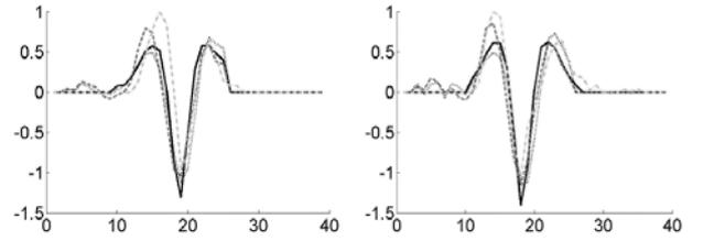
FIG. 1: The MUAPs decomposed from synthetic surface EMG signals (3 active MUs) by our HOC-based method. The original MUAPs are depicted solid, the decomposition results in the noise-free condition dashed, the results at SNR = 10 dB dotted and at SNR = 0 dB dash-dotted.
