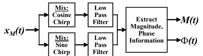
FIG. 2: Overview of mixing technique. Measured input  $x_M(t)$  is the excitation chirp wave, modified by the frequency response of the analog signal conditioning circuit, plus measurement noise. The mixing technique produces an estimate of the measured chirp magnitude  $M(t)$  and phase  $\Phi(t)$  at each time index  $t$ .
