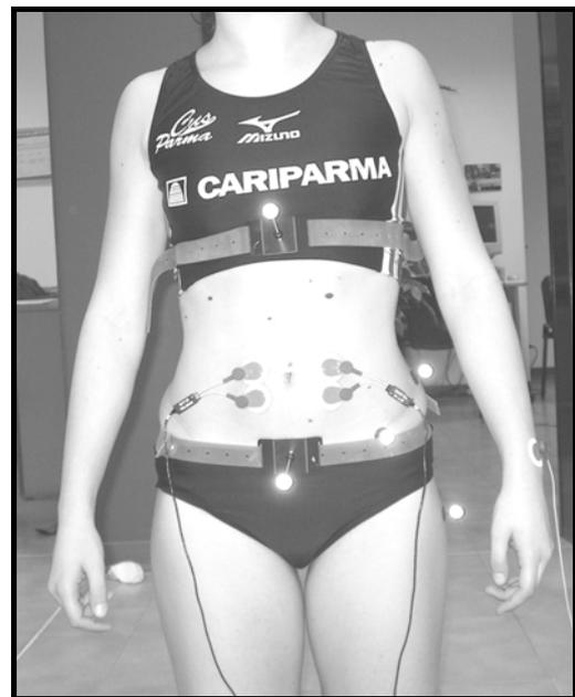
FIG. 1 : Surface electromyographic electrode arrangement, front view.
