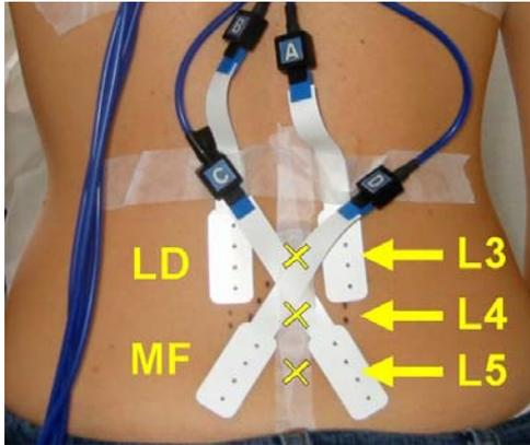
FIG. 1: Detail of the experimental set-up for surface EMG signal detection. Four adhesive electrode arrays (four electrodes, 10 mm inter-electrode distance) were located on the Longissimus Dorsi (LD) and Multifidus (MF) muscles, at the level of the lumbar vertebrae L3 and L5 respectively, aligned with the fiber direction.
