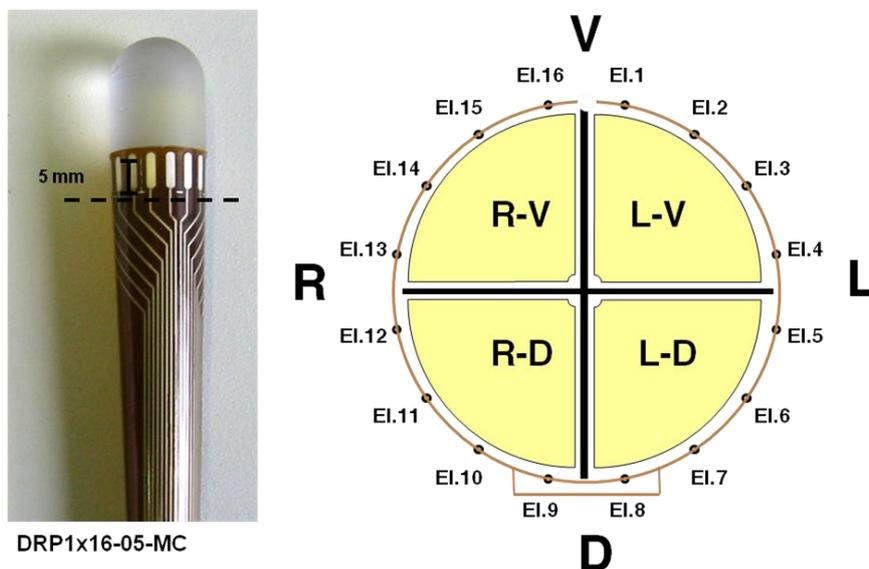
**Figure 5.** Rectal probe used in the TASI-2 project and schematic image of the probe section with the indication of electrode numbers and the four quadrants (Left Ventral - LV, Left Dorsal - LD, Right Dorsal - RD, Right Ventral - RV).
