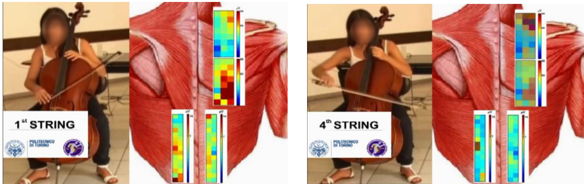
Fig. 5. Surface EMG activity of the right trapezius and of the lumbar erector spinae in a cello player playing the first and the fourth string of the cello. Longitudinal differential detection. Electrode array of 12 rows by 5 columns. Interelectrode distance = 8 mm. The images represent the RMS of the sEMG of each pixel (electrode pair) computed on an epoch of 125 ms and provide information about the time evolution of the activity of the muscles under the electrode grids. See related videos on www.robertomerletti.it -> Teaching material(clinical) -> Videos -> N.15-19.
